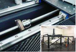
Autoscale's CNC technology (inset), which cuts objects up to 16 feet long, benefits from Thomson linear components, including precision ball screws and a profile rail that proved to be the only one long enough to meet their system requirements.
