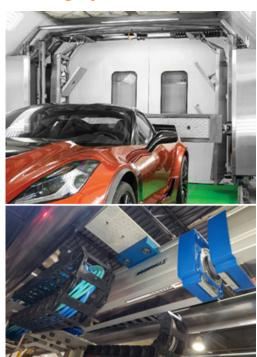
The Movopart units attach to the system's stepper motors via Thomson RediMount™ motor mounting adapter kits, which enable seamless installation in only a few minutes.
